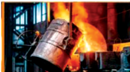
MELTING – 3 NOS (3 TON / 3TON & 0.5 TON) MEDIUM FREQUENCY INDUCTION FURNACE
